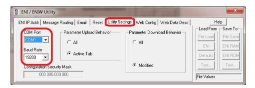
**STEP #9** — Select the "ENI IP Addr" tab. Next, set the 232 Baud Rate to "Auto." Set the IP address of the 1761-NET-ENI. Ensure the ENI series is correct. Provide the "ENI IP Address", "Subnet Mask" and "Gateway" where necessary.
